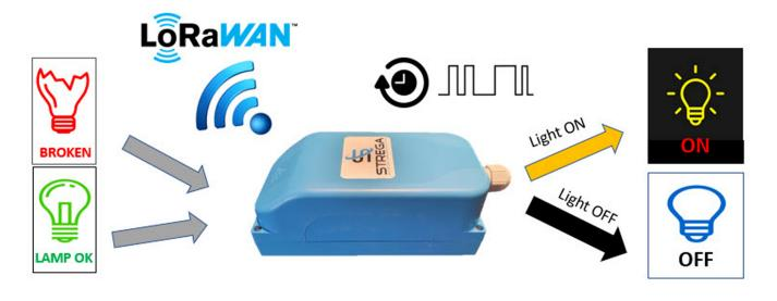
The STREGA time-controlled Emitter is a long distance wireless switching device with embedded **LoRaWAN®** technology. With its ultra-low-power consumption, the Smart-Emitter can trigger ON or OFF operations from its embedded AC bistable relay that can feed street light poles or feeders. The emitter is working on external power (Class C) or on batteries during 7+ years (Class A) and through extreme long distances with exceptional obstacles penetration.
